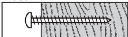
If your wall is solid wood use any of the FIXA screws, no plug is needed in most cases and it is not necessary to pre-drill. A rule of thumb is that the length of the screw should be twice as long as the thickness of the object you intend to install onto the wooden wall.
