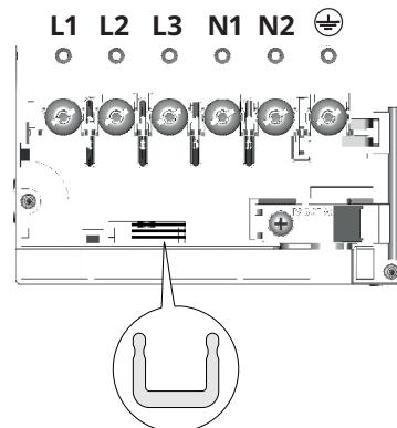
Insert the shunts between the screws as shown
